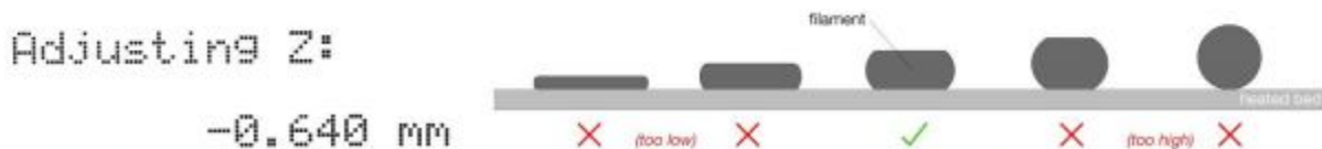
Pict. 10 - How to tune the nozzle height live during the test print. Note: -0.640 mm is only for illustration. Your setting will be different!
